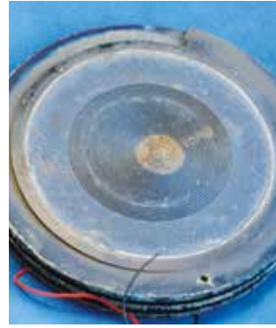
Figures 6 and 7: Large-scale discoloration of the coating surface.
