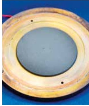
Figures 6 and 7: Large-scale discoloration of the coating surface.
