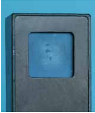
Figure 5: Local overheating of a photodiode sensor.
