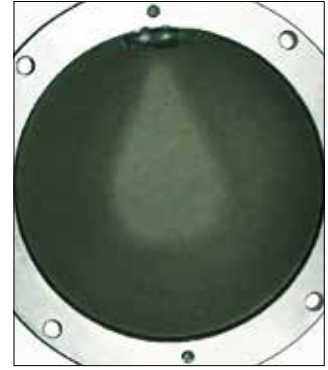
Figure 8: Example of grease contamination just from overheating.
