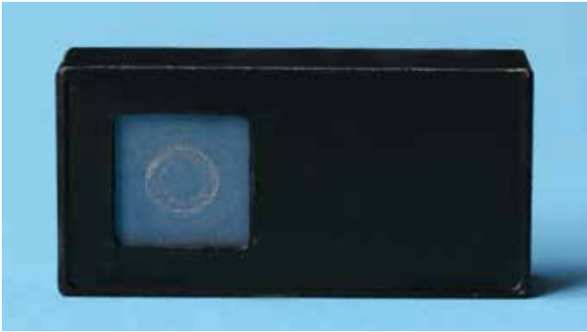
Figure 9: Overheating of photodiode sensors can cause burn spots or discoloration of the coating surface.
