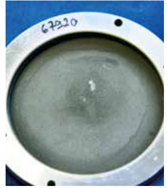
Figures 3 and 4: Local overheating directly results in burn marks. Usually, it is the discs that need to be replaced.
