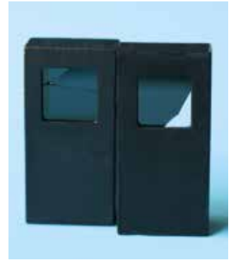
Figures 10 and 11: Photodiode sensors must be handled with care; otherwise they can crack.
