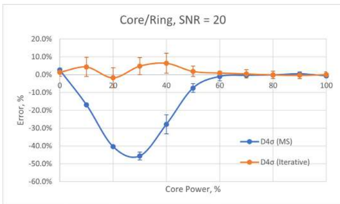
Figure 6 - Error of Beam Width Measurement as a Function of Core Power
