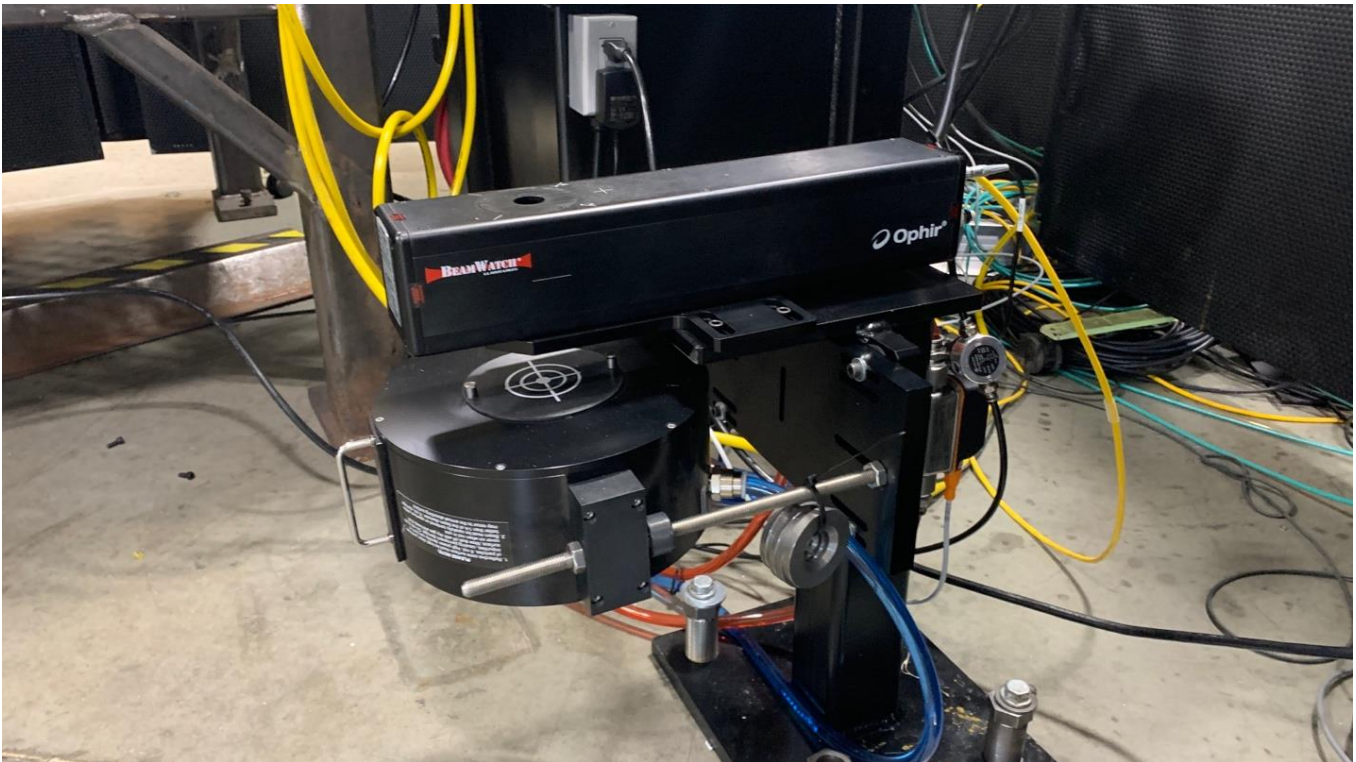
Figure 4. An Ophir BeamWatch beam profiler is coupled with a 30K-W sensor and used for characterizing the beam offline and at-process in a laser welding cell.
